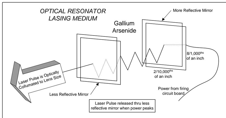
The atoms of the lasing medium are put into an excited state by an external energy source (e.g., the power from a firing circuit board). Some of this energy is stored by the atoms. As the atoms become excited, they are stimulated to release the stored energy as light energy resulting in amplification of incoming light.
